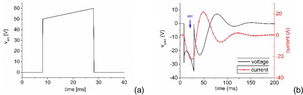
**Fig. 6: (a) Voltage waveform of the arc generator, (b) computed transient oscillation of voltage and current triggered by the arc voltage profile**
