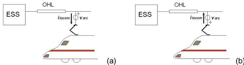
Fig. 4: Direction of the voltage drop emulating the arc for (a) traction and (b) braking phases
