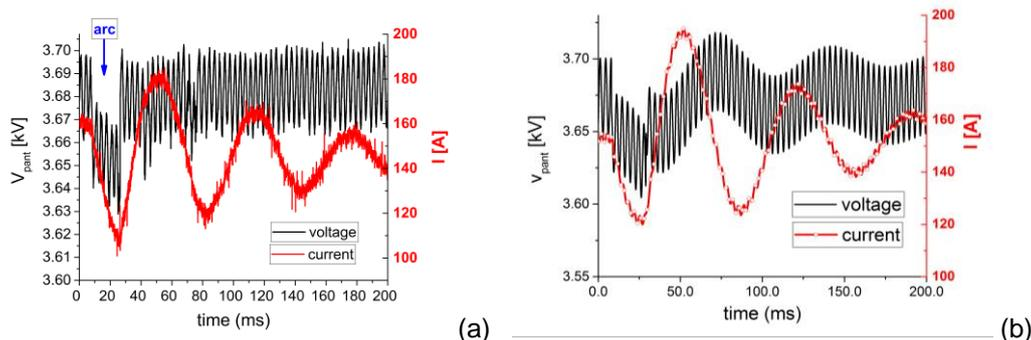
**Fig. 7: (a) Measured and (b) simulated conducted effects of arc event**
