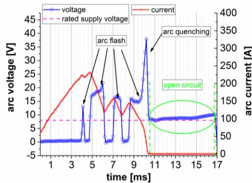
Fig. 3: Time behavior of arc voltage and current during the random arc events.
