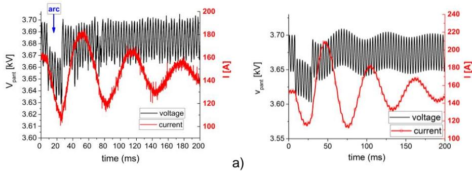
**Fig. 8: (a) Measured and (b) simulated conducted effects of arc event (no ESS filter)**
