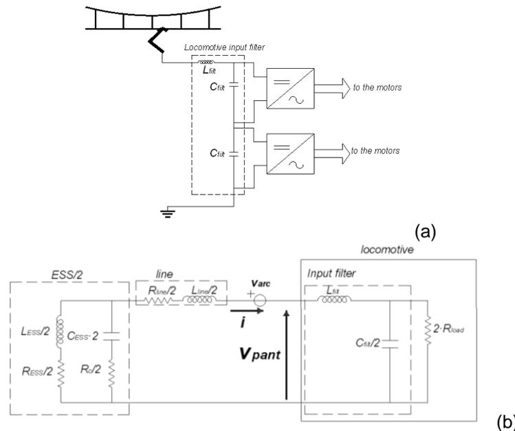
Fig. 5: (a) E464 input filter and traction system, (b) simplified equivalent circuit.
